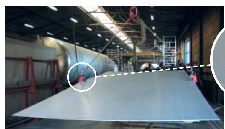
TURNING AND VERTICAL TRANSPORT STEEL PLATE - STEEL CONSTRUCTION COMPANY
