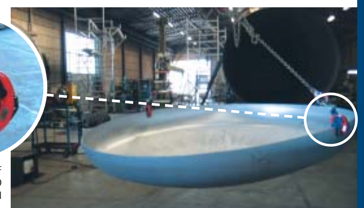
HORIZONTAL TRANSPORT STAINLESS STEEL PLATE - CHEMICAL EQUIPMENT MANUFACTURING
