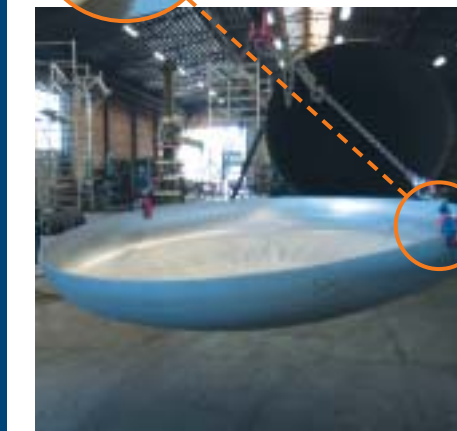
HORIZONTAL TRANSPORT OF STAINLESS STEEL VESSELHEAD / VESSEL- AND VESSELHEAD PRODUCTION
