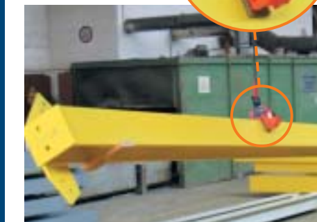
TRANSPORT OF PAINTED H-BEAMS / HALL- AND CONSTRUCTION BUILDING
